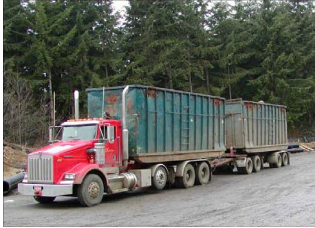
Figure 3-5- Truck with dual chip bin trailers loaded with chips 2
