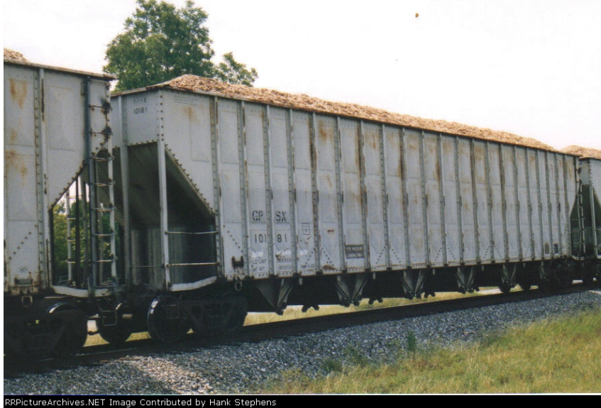
Figure 3-16- Open top hopper with bottom discharge, GPSX 9
