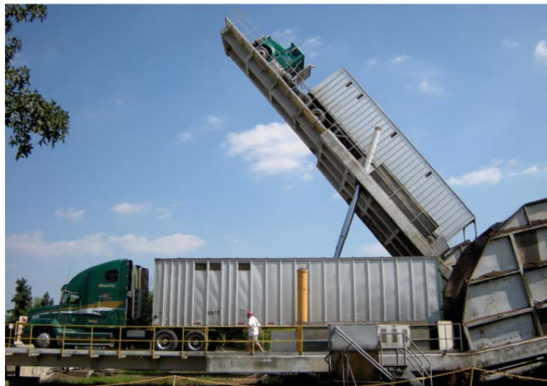
Figure 3-8- A type of chip truck tipper at a woody biomass facility (Jeuck, 2009)
