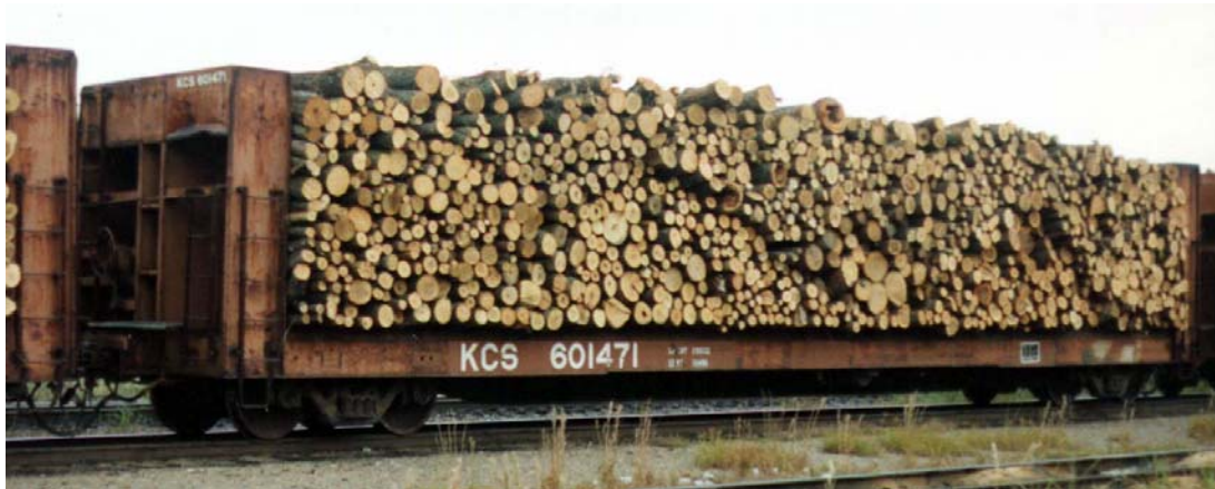
Figure 3-13. Bulkhead car-Kansas City Southern Railway 6
