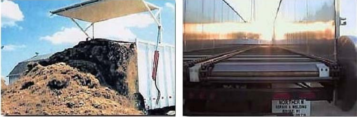
Figure 3-9- Left: walking floor truck during unloading; Right: inside of walking floor truck 5
