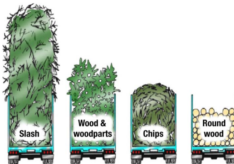
Figure 3-1- Different size capacity of materials with same weights (Schroeder et al, 2007)
