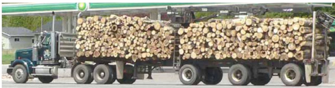
Figure 3-3- Tractor-trailer combination with self-loader capability (Green et al. 2005)
