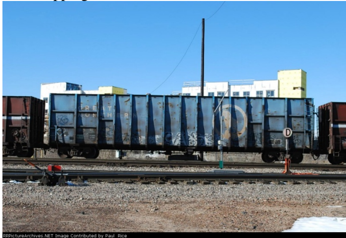
Figure 3-15. Woodchip gondola with front and rear gates, Great Northern 8
